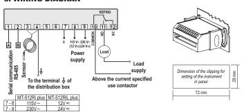
Note: The length of the sensor cable may be increased by the user up to 200 meters, using a 2 x 24 AWG cable. For immersion in water, use thermometric well.
